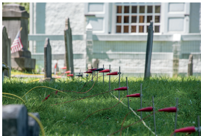
Looking north towards the historic church, a segment of the resistivity electrodes comprising one of six lines are shown in this compressed image. Courtesy of Roger D. Thorne.
