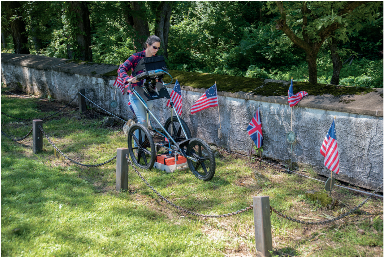
Dr. Laura Sherrod pushes the GPR control unit through the traditional burial plot during the first geophysical survey at St. Peter's churchyard, June 11, 2019. Courtesy of Roger D. Thorne.
